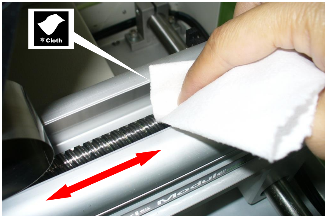
Step 4: Wipe the old grease away from the ball screw.
