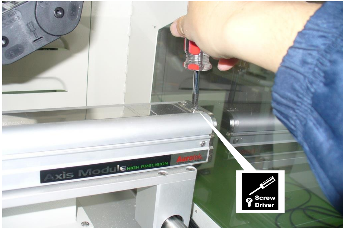
Step 7: Reinstall the silicon steel sheet.
