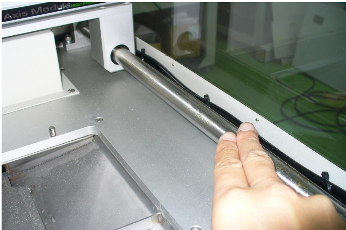
Step 4: Averagely smear new grease on the ball screw.
