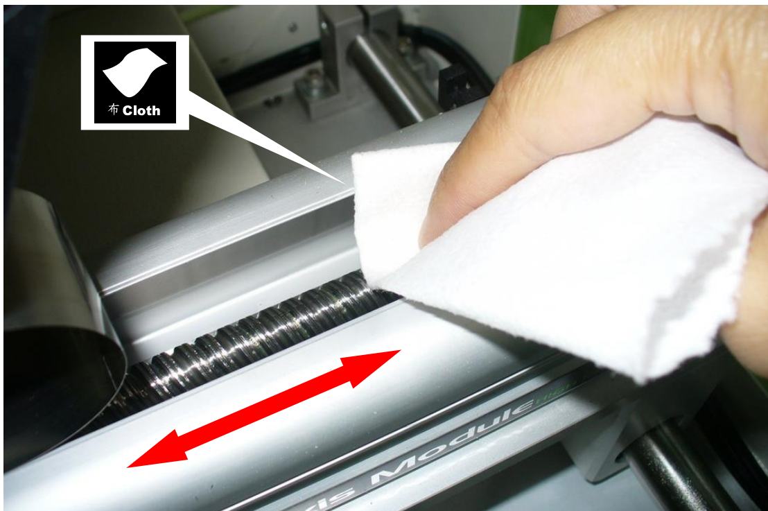
Step 6: Wipe the excess grease away to prevent dust adhesion.
