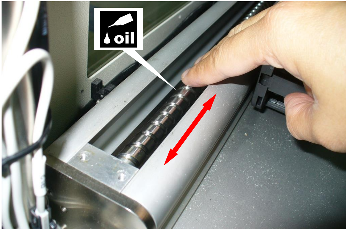
Step 5: Averagely smear new grease on the ball screw.
