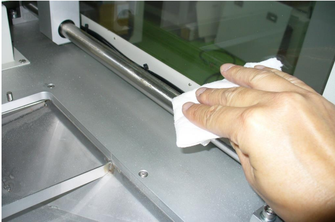
Step 5: Wipe the excess grease away to prevent dust adhesion.
