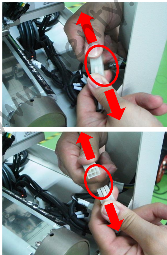
Step 3: Remove X axis/Y axis motor power cable.
