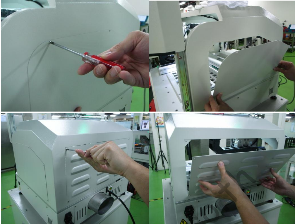
Step 2: Remove the covers.
