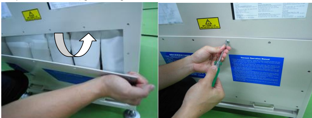
Step 7 : Close and lock the filter cover.
