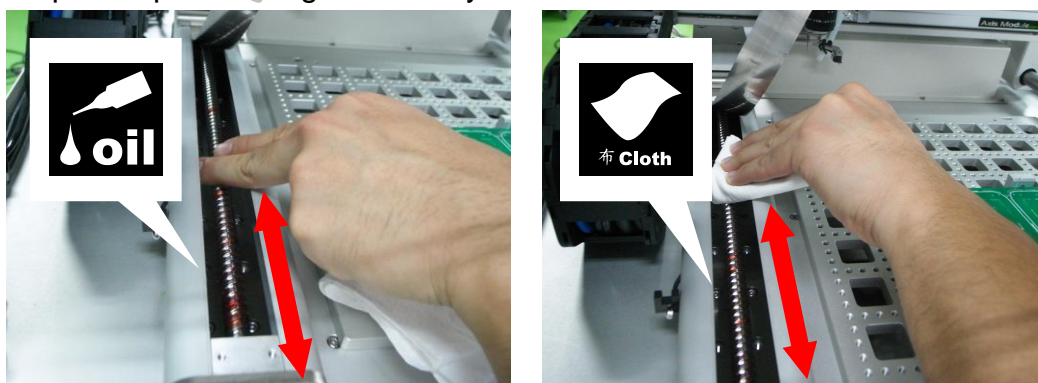
Step 7: Averagely smear new grease on the ball screw and wipe the excess grease away to prevent dust adhesion.
