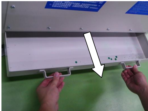
Step 5 : Pull out the dust drawer, use vacuum cleaner to clean the dust.
