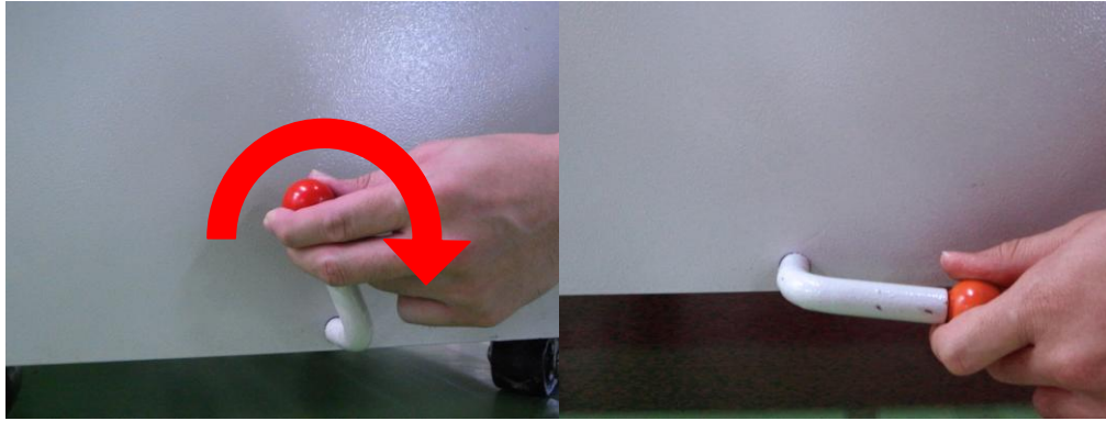
Step 4 : Release dust gathering drawer Locker lever.
